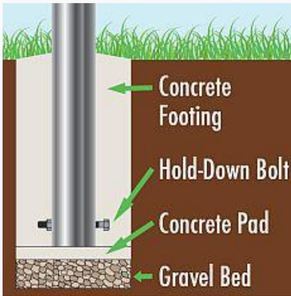
Lay a 4inch (100mm) depth of 3/4inch diameter gravel at the base of the hole. Next, pour a 4inch (100mm) depth of concrete to provide a solid pad. Patio stones can be substituted in place of the poured concrete. Insert the post with a hold down bolt through the post to keep it secure. (see diagram) Pour the concrete footing and temporarily brace the posts until the concrete has set.
